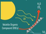
**Airborne pollutants** such as VOCs can be **transformed into harmless compounds** (H<sub>2</sub>O and CO<sub>2</sub>).
